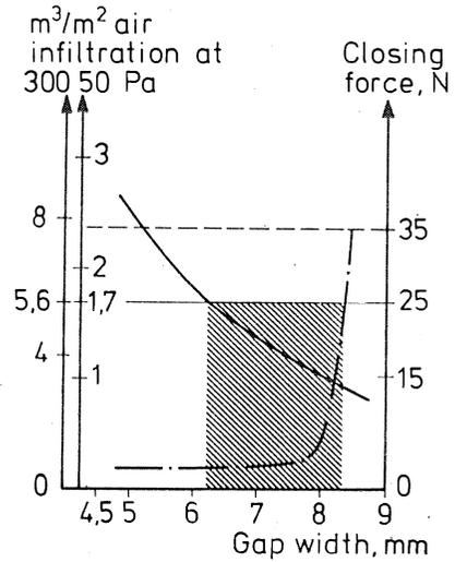
Figure 2. Tubular strips (h=10 mm, t=0.8 mm).
