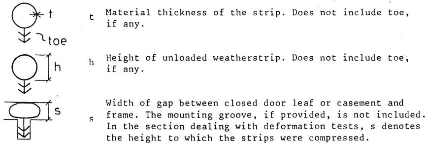
*The performance range of the strip.* This is the range, bounded by two values of *s*, over which a weatherstrip satisfies the requirements specified with regard to airtightness and closing force.
