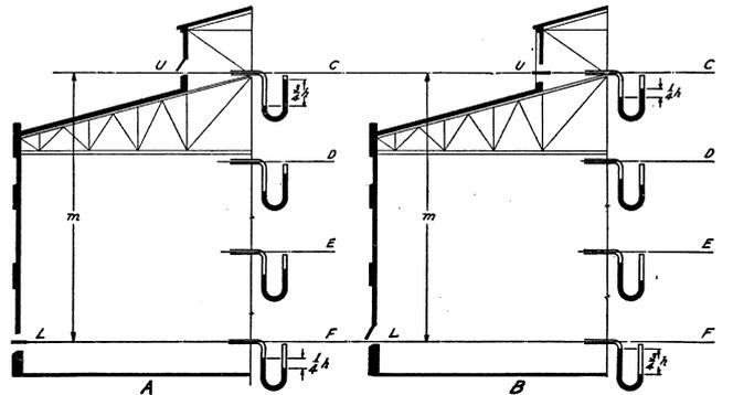
FIG. 3. PRESSURE RELATIONS WHEN OPENINGS "U" AND "L" ARE OF UNEQUAL AREAS
