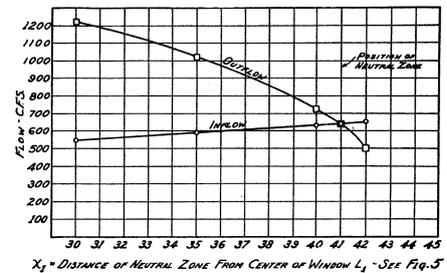
FIG. 6. PLOTTING OF VALUES OF FLOW FOR VARIOUS ASSUMPTIONS OF TABLE 1 TO FIND THE POSITION OF THE NEUTRAL ZONE
