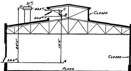
FIG. 7. SECTION THROUGH FOUNDRY AT UNIVERSITY OF MICHIGAN SHOWING AREAS AND VERTICAL DISTANCES
