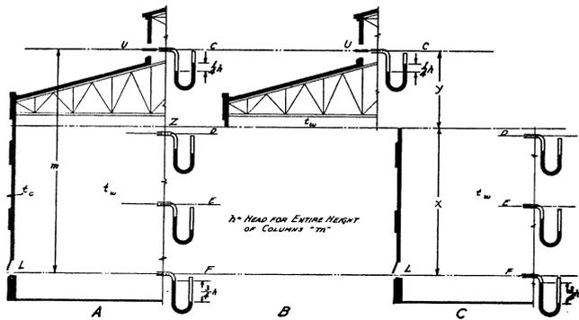
FIG. 4. SHOWING HOW THE TOTAL HEAD IS DISTRIBUTED TO UPPER AND LOWER OPENING IN PROPORTION TO THEIR DISTANCE FROM THE NEUTRAL ZONE
