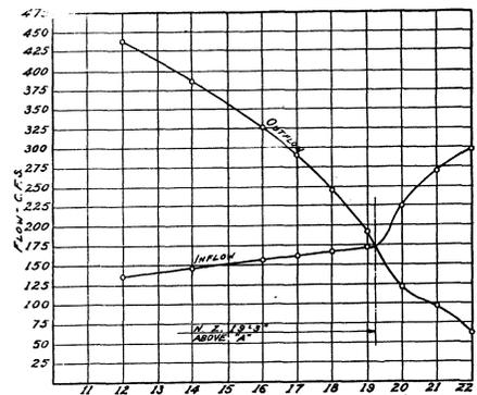
FIG. 8. PLOTTING OF VALUES OF INFLOW AND OUTFLOW FOR VARIOUS ASSUMPTIONS OF TABLE 3 TO FIND POSITION OF THE NEUTRAL ZONE
