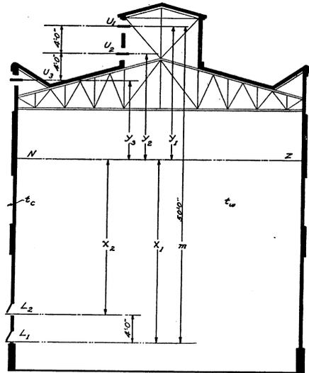
FIG. 5. ILLUSTRATING CASE OF SEVERAL OPENINGS AT VARIOUS LEVELS
