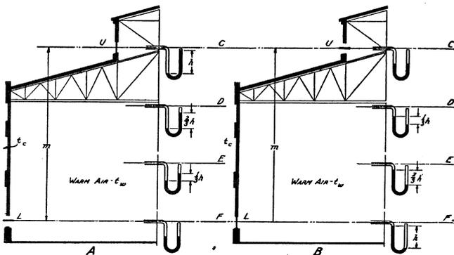
FIG. 1. WARM-AIR COLUMNS PLACED IN ATMOSPHERE OF COOL AIR; SHOWING DIFFERENCE IN PRESSURES WHEN A SINGLE OPENING AT TOP OR BOTTOM IS PROVIDED AS INDICATED BY LIQUID IN GAGES. NO FLOW OCCURRING
