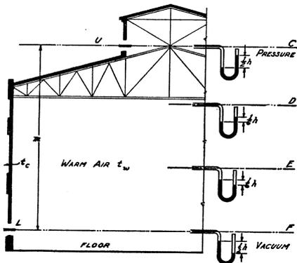
FIG. 2. ILLUSTRATING PRESSURE RELATIONS WHEN "U" AND "L" ARE OF EQUAL AREA, AND FLOW RESULTS FROM TEMPERATURE DIFFERENCE
