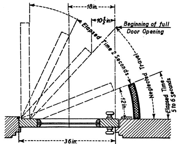
FIG. 1. DIAGRAM SHOWING MEASUREMENT OF EFFECTIVE DOOR OPENING.
