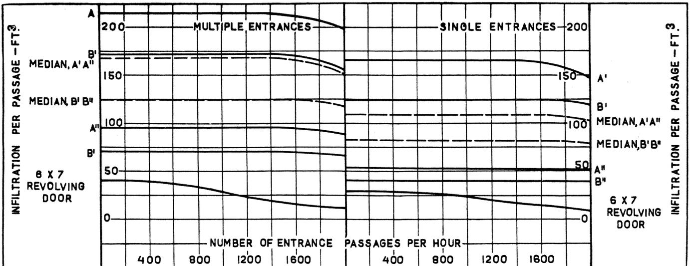
FIG. 4. COOLING LOAD LOSSES DUE TO DOOR FILTRATION IN MULTIPLE AND SINGLE ENTRANCE BUILDINGS.
