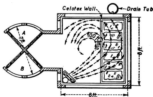
FIG. 2. PLAN OF REVOLVING DOOR TEST BOOTH.
