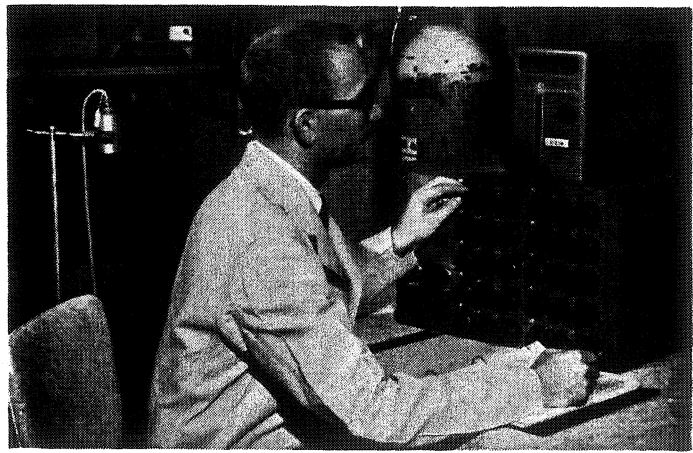
Fig. 3 Portable air infiltration meter console. Sensing probe is shown at left
