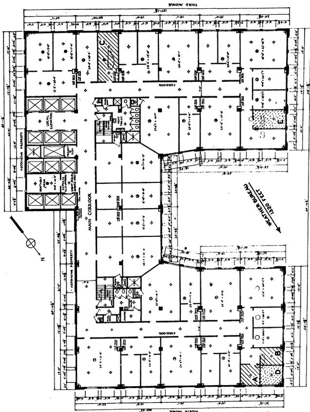
FIG. 2. PLAN OF FOURTH TO TWENTY-THIRD FLOORS OF GRANT BUILDING SHOWING ROOMS A, 705; B, 707; C, 726 AND 1825. ROOMS 2703, 2706, 2715, AND 2718 ARE SIMILARLY SITUATED TO A, D, E, AND C, RESPECTIVELY, BUT SET BACK FROM THE BUILDING
