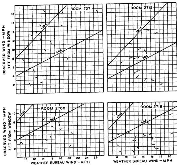
FIG. 4. RELATION BETWEEN OBSERVED WIND 3 FT FROM WINDOW AND WIND RECORDED BY WEATHER BUREAU. ALL DATA FOR A NORTHWEST WIND AT WEATHER BUREAU. ARROW POINTS INDICATE MAGNITUDE AND DIRECTION OF WIND TO OBSERVER FACING WINDOW FROM WITHIN. LINES INDICATE OBSERVED WINDS OF 100 PER CENT AND 50 PER CENT OF WEATHER BUREAU VELOCITIES
