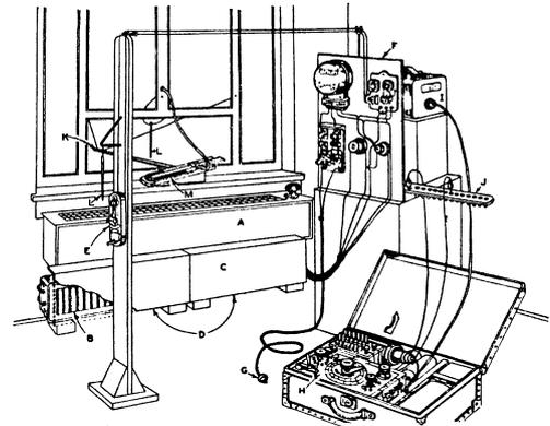
FIG. 3. TEST ROOM SHOWING HEATER AND TEST EQUIPMENT
