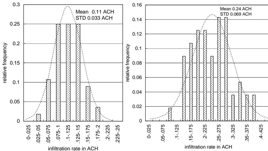
Figure-11(a) Distribution of estimated infiltration rate for the post and beam construction method (2 storied wooden detached houses) for summer (left) and winter (right)
