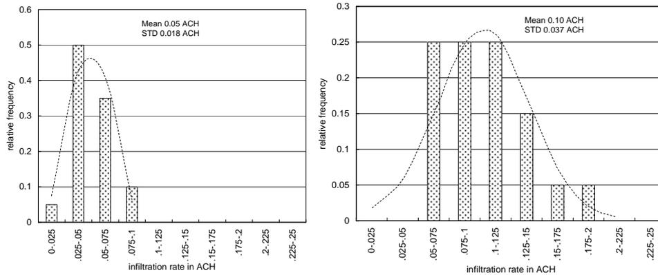
Figure-11(b) Distribution of estimated infiltration rate for the two-by-four construction method (2 storied wooden detached houses) for summer (left) and winter (right)
