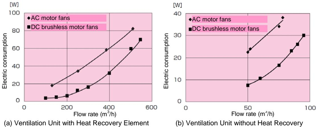
Figure 12 - Comparisons of Electric Consumption of Ventilation Equipment with AC and DC Fans
