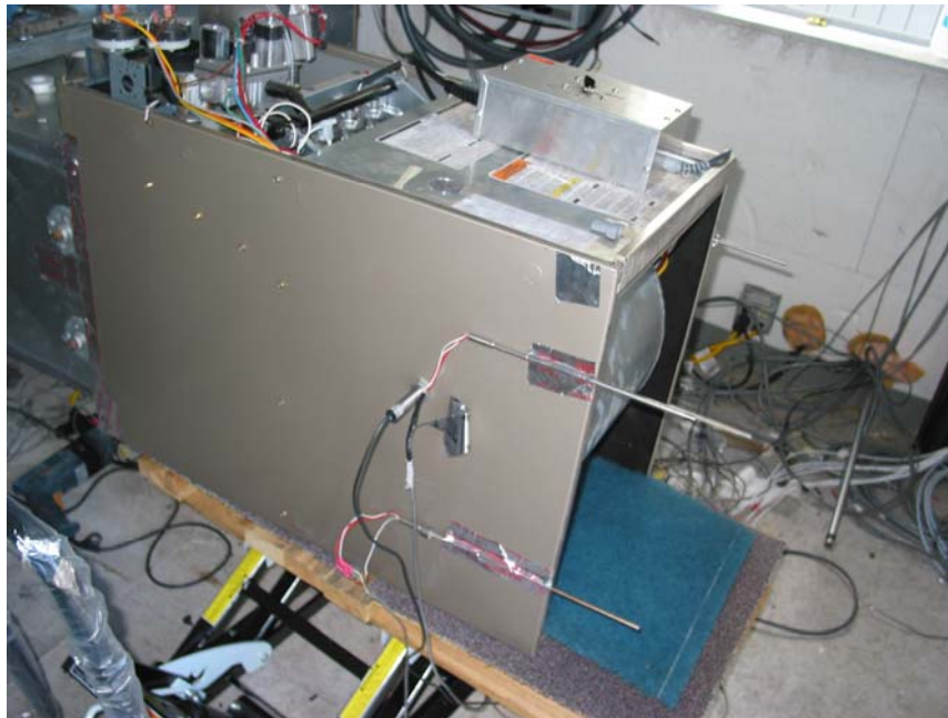
Figure 13. Furnace mounted in electric utility test apparatus
