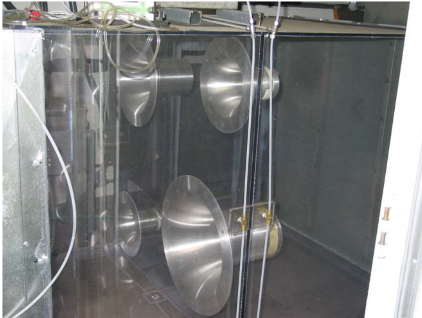
Figure 14. Flow nozzles in electric utility test apparatus
