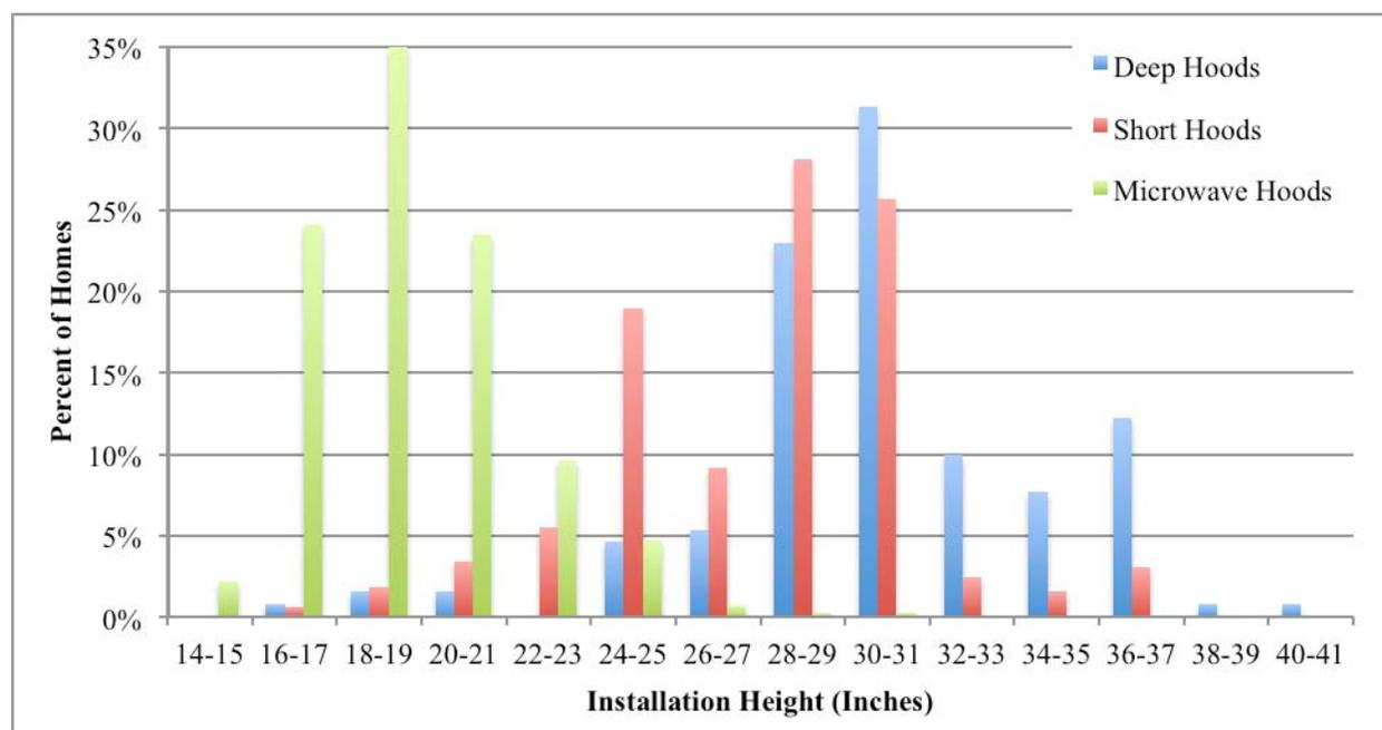
**Figure 15. Installation height by type of range hood.**
