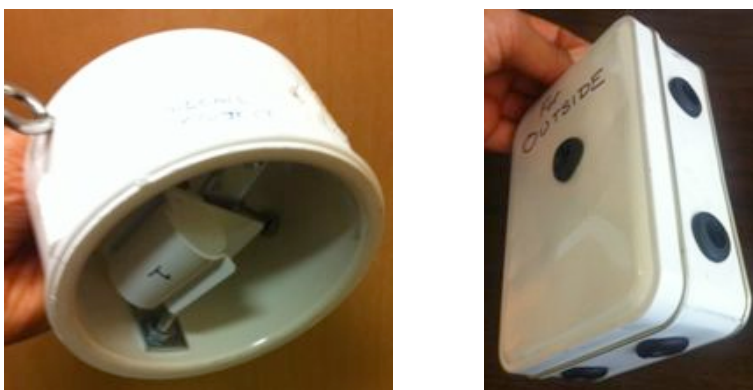
Figure 2.3. Two enclosure configurations for \text{NO}_2 / \text{NO}_x sampling: Configuration on the left was used at homes that were visited and has been validated in past studies. Configuration on the right was used at homes to which samplers were mailed.
