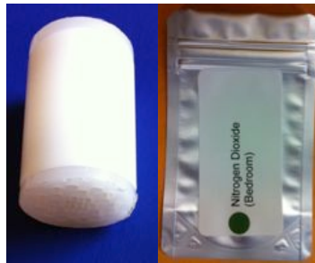
Nitrogen dioxide sampler inside airtight bags
