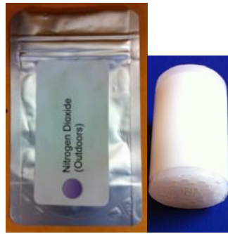
Nitrogen dioxide sampler inside airtight bag
