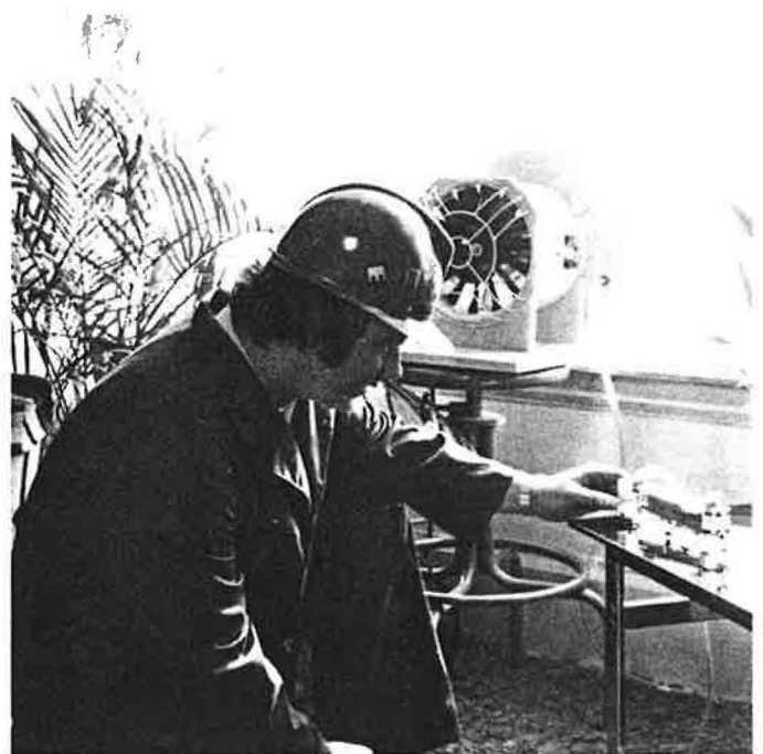
FIGURE 3 — Fan equipment for air-leakage tests.
