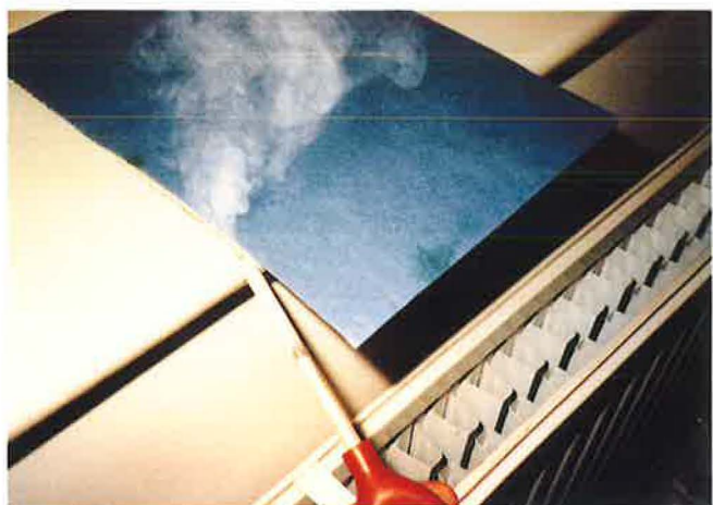
Simple observation with a smoke pencil
