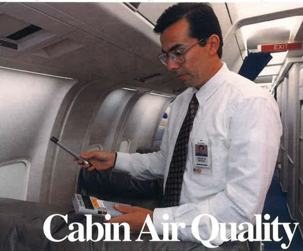
Boeing Engineer taking relative humidity measurements
