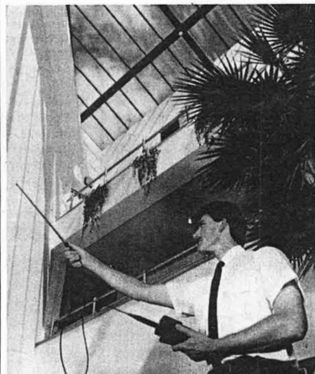
Airflow can be effectively measured by monitoring carbon dioxide. This gas is exhaled by all occupants, making it representative of the ventilation needs of an occupied zone.
