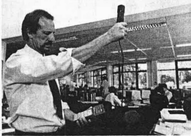
Monitoring ventilation rate in an office atrium - ensuring an adequate ventilation rate to sweep away airborne contaminants is widely seen as more effective than monitoring indoor air quality.
