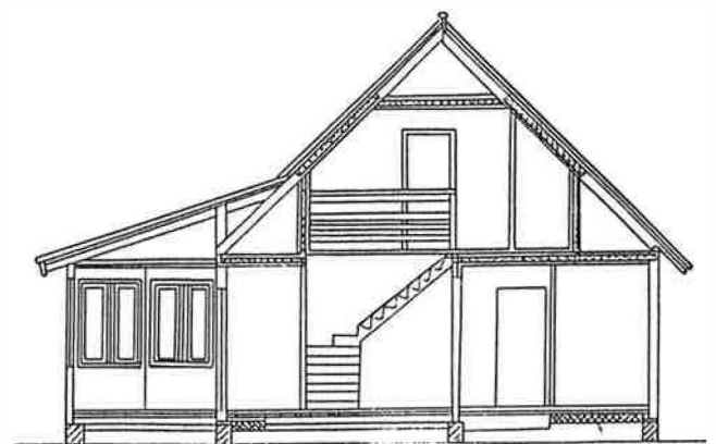
Fig. 1. Section of the house examined.
