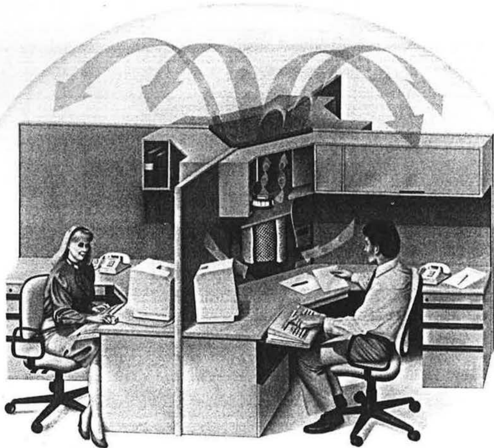
Fig. 3 Diagram of the pattern of air circulation with a furniture-integrated BZF system.
