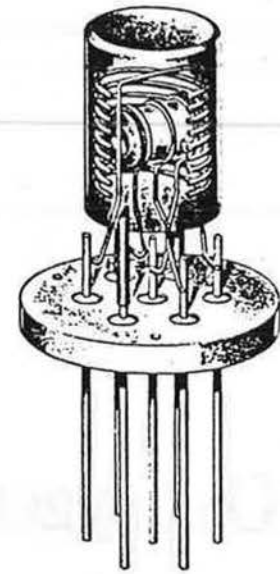
Fig.1 Cutaway view of the oxygen sensor. Two zirconium oxide discs with porous platinum electrodes attached to a platinum ring enclose a small chamber, see Fig.2. Surrounding the disc and ring assembly is a heating coil. Unlike other oxygen sensors, this sensor requires no reference gas or 'calibrated leak'
