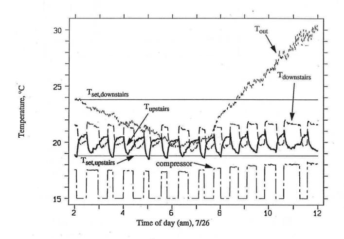
FIGURE 2. Upstairs cooling only, room temperature response and outside temperature, °C, rescaled compressor power demand showing system operation.  $T_{\text{set,up}}$  =18.8 °C,  $T_{\text{set,down}}$  = 23.8 °C  $T_{\text{up}}$  = 19.8 °C,  $T_{\text{down}}$  = 20.7 °C
