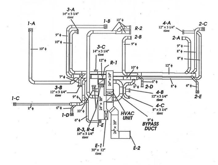
Figure A4. Duct system layout, location is between floors (not to scale). Register dimensions in accompanying table.
