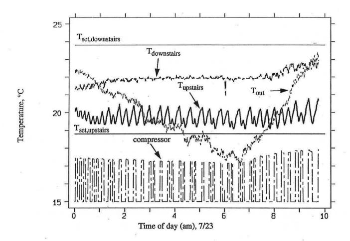
FIGURE 5. Master bedroom cooling with installed zone separation, room temperature response and outside temperature, °C, rescaled compressor power demand showing system operation.  $T_{\text{set,up}} = 18.8$  °C,  $T_{\text{set,down}} = 23.8$  °C,  $T_{\text{up}} = 19.7$  °C,  $T_{\text{down}} = 22.0$  °C
