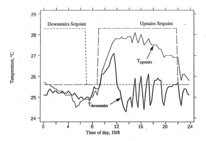
FIGURE 3. Downstairs cooling only, room temperature response, upstairs and downstairs thermostat schedules, average temperatures between 9 am and 10 pm:  $\overline{T}_{up} = 27.4$  °C,  $\overline{T}_{down} = 25.5$  °C
