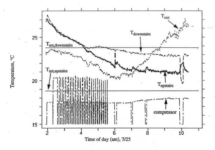
FIGURE 4. Master bedroom cooling only, room temperature response and outside temperature,  $^{\circ}$ C, rescaled compressor power demand showing system operation.  $T_{\text{set,up}} = 18.8 \,^{\circ}$ C,  $T_{\text{set,down}} = 23.8 \,^{\circ}$ C,  $T_{\text{up}} = 21.1 \,^{\circ}$ C,  $T_{\text{down}} = 22.7 \,^{\circ}$ C
