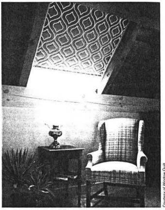
The Window Quilt skylight covering shown here cuts down on energy losses at night.
