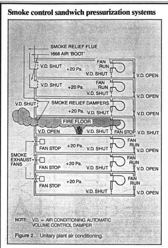
of these dampers, or the unitary plant, that achieves the necessary pressure differentials between floors.
