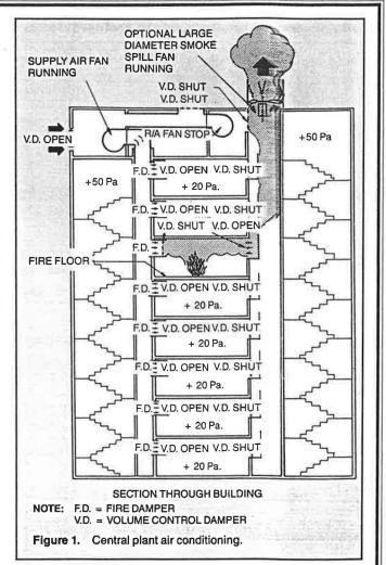
Non-fire floor pressurization is achieved by operating the airconditioning system at 100% fresh air.
