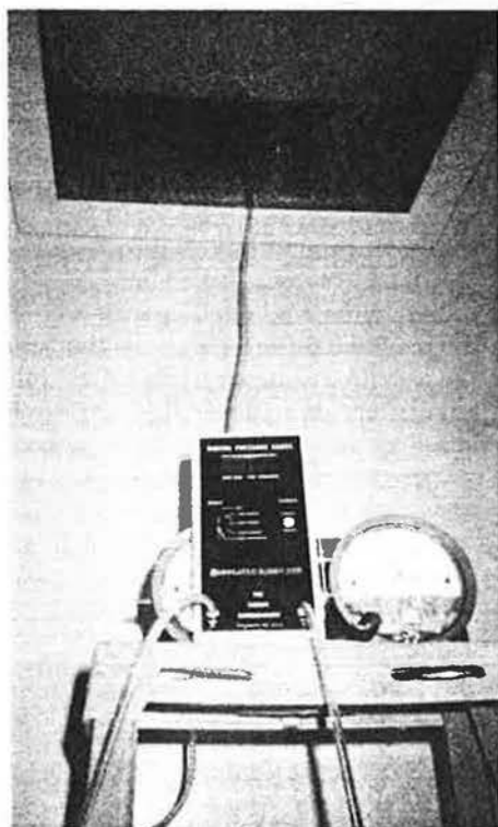
"Opening a door" to air leakage measurements, this method of testing is simple. Visible here are the gauges measuring pressure across an open attic door.
