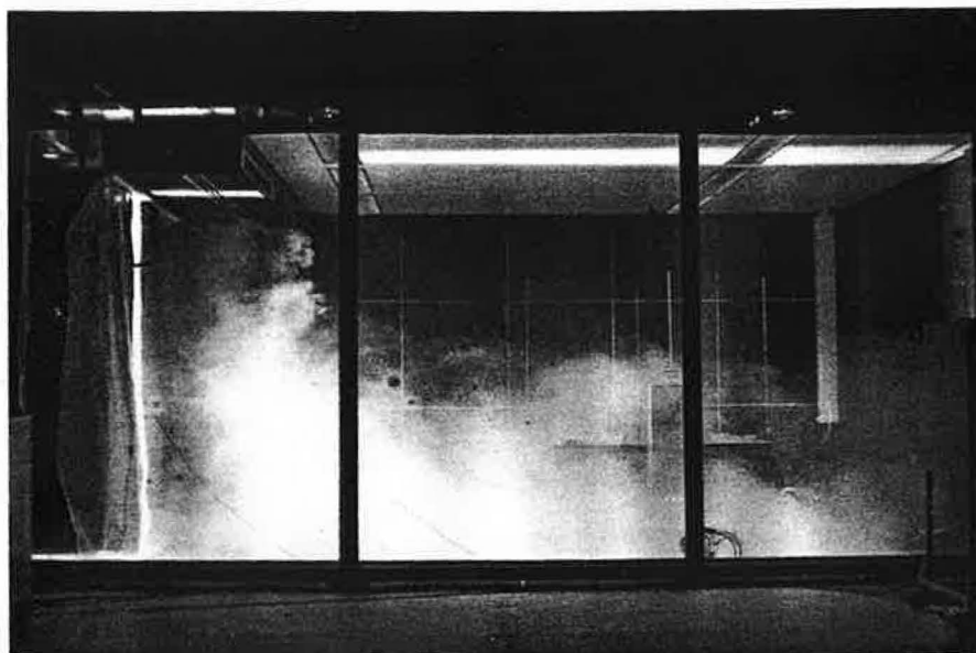
Figures 2a & 2b: Illustration of the air flow regimes by means of smoke trace (overall cooling load of 50\text{ W/m}^2 , and primary air at 50\text{ m}^3/\text{h} ).
