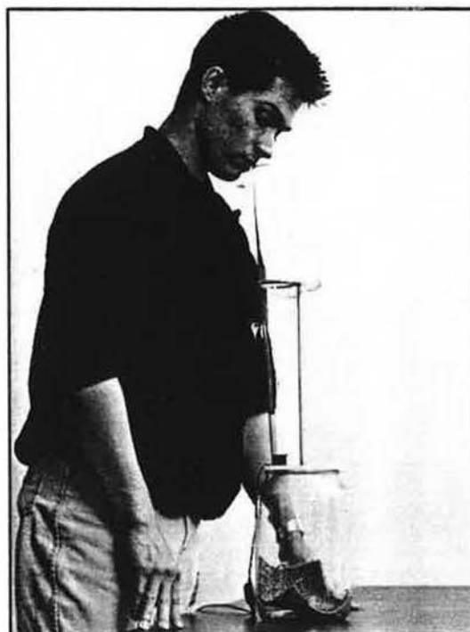
Fig. 4 A trained panel member evaluating a pollution source at the bottom of the jar.
