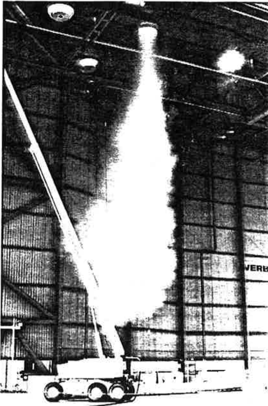
Fig. 18. Low turbulent air supply from 26 m height in a heating mode
