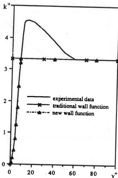
Figure 5 Wall function for turbulent kinetic energy
