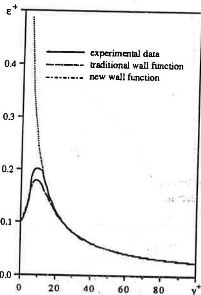
Figure 6 Wall function for dissipation rate
