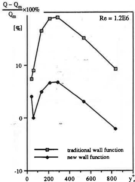
Figure 9 Variation of total heat transfer with the distance of near-wall mesh, Case 3
