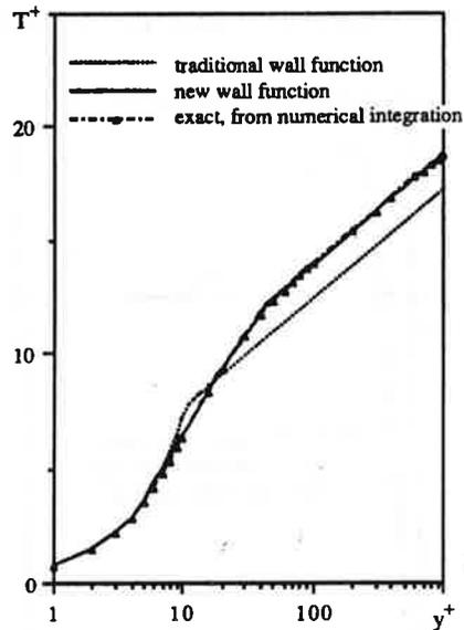
Figure 4 wall function for temperature
