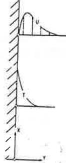
Figure 1 Velocity and temperature profile near a heated wall
