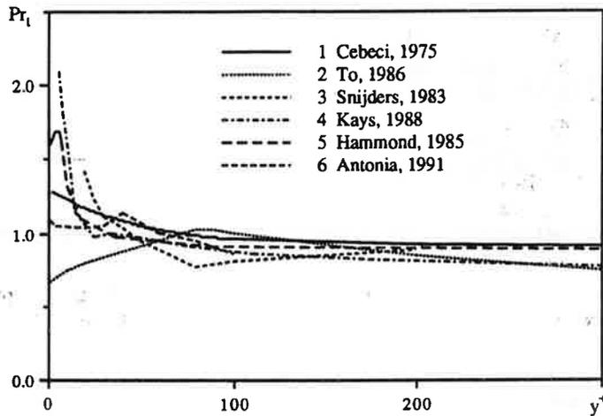
Figure 2 Turbulent Prandtl number functions
