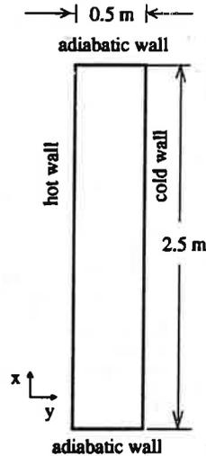
Figure 10 Sketch of the air-filled cavity, Ref. [29]
