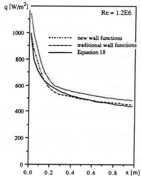
Figure 8 Comparison of local heat flux with measurement for Case 3
