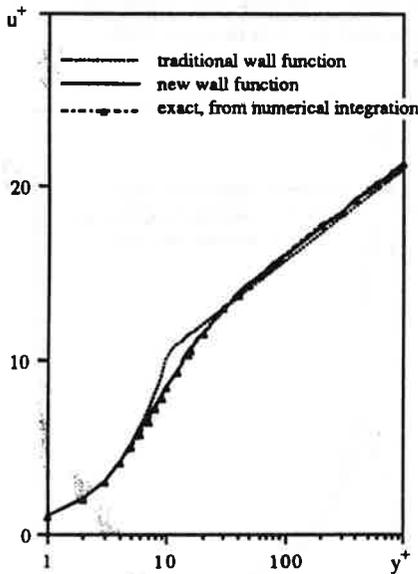
Figure 3 Wall function for velocity
