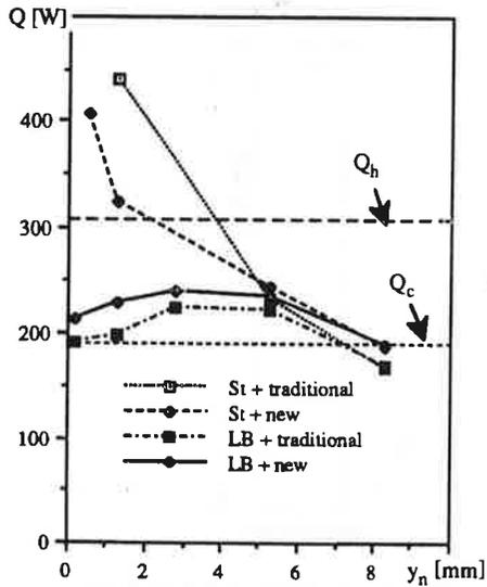
Figure 11 Variation of total heat transfer with the distance of near wall grid
