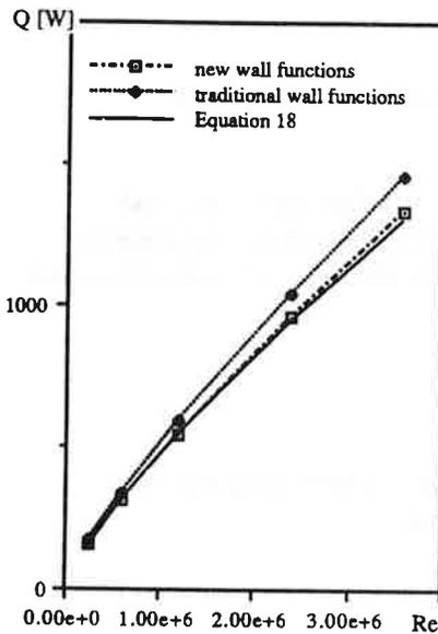
Figure 7 Comparison of total heat transfer with measurement
