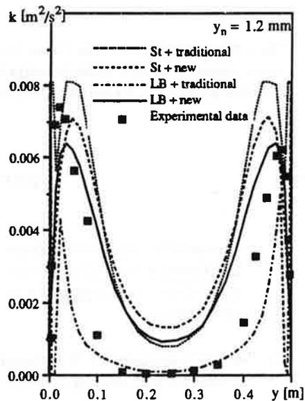
Figure 15 Profiles of turbulent kinetic energy at half-height
