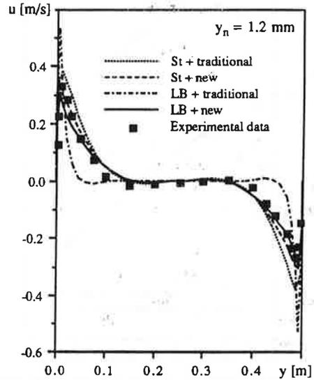
Figure 12 Profiles of vertical component of velocity at half-height
