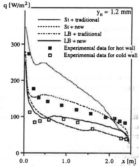
Figure 14 Profiles of local heat flux on vertical wall
