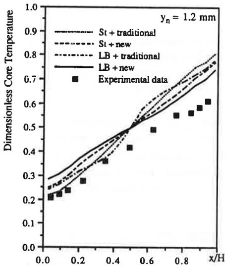
Figure 13 Vertical temperature profiles in the mid-section
