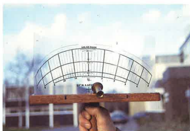
Fig 10 Instrument for measuring horizon profile ('solar site selector')
