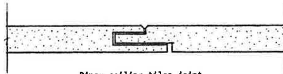
Pinex ceiling tiles joint
