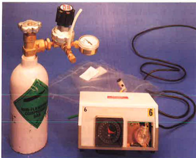
Figure 2 BRESIM equipment — gas bottle, sampler unit and bags
