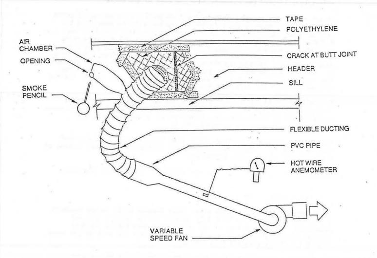
This test methodology made it possible to have a great deal of sensitivity in monitoring the relative pressures and adjusting the flow from the crack chamber.
