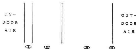
Fig. 1. The structure of the wall. ① Fiberboard, 5 mm; ② insulation, 5 cm; ③ ALC, 10 cm; ④ water barrier.
