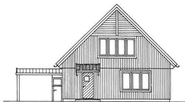
Fig. 3. The picture above shows the house facades facing the street. The facades are of vertical wooden boarding. On the left, a cross-section of the house construction. The houses are prefabricated to a fairly high degree. The foundation elements, which are left in position, act as forms for the concrete slab which is cast on the spot. These foundation elements consist of a core of polystyrene foam surrounded by an outer layer of concrete reinforced with steel fibre and glassfibre
