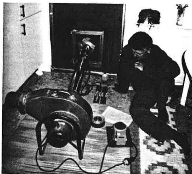
Fig. 7. Measurement of the air leakage rate.
