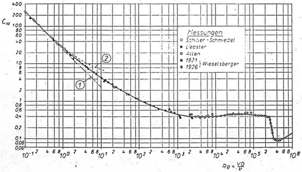
**Fig. 2** Drag coefficient ( $C_w$ ) of a sphere as function of Reynolds number (based on diameter  $D$ ).
