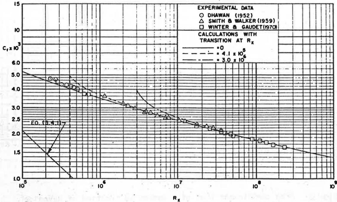
Fig. 4 Local skin-friction coefficient on a smooth flat plate.
