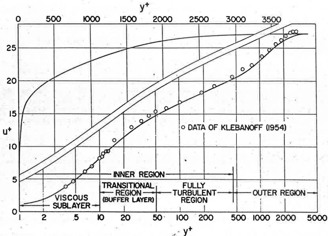
**Fig. 5** Semi-logarithmic and linear plots of mean velocity distribution across a turbulent boundary layer with zero pressure gradient. The linear plot is included to show a true picture of the thickness of various portions.
