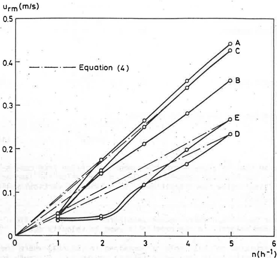
**Fig. 6** Maximum velocity in the occupied zone as a function of the air exchange rate. The tests were performed for five different air terminal devices (A to D)
