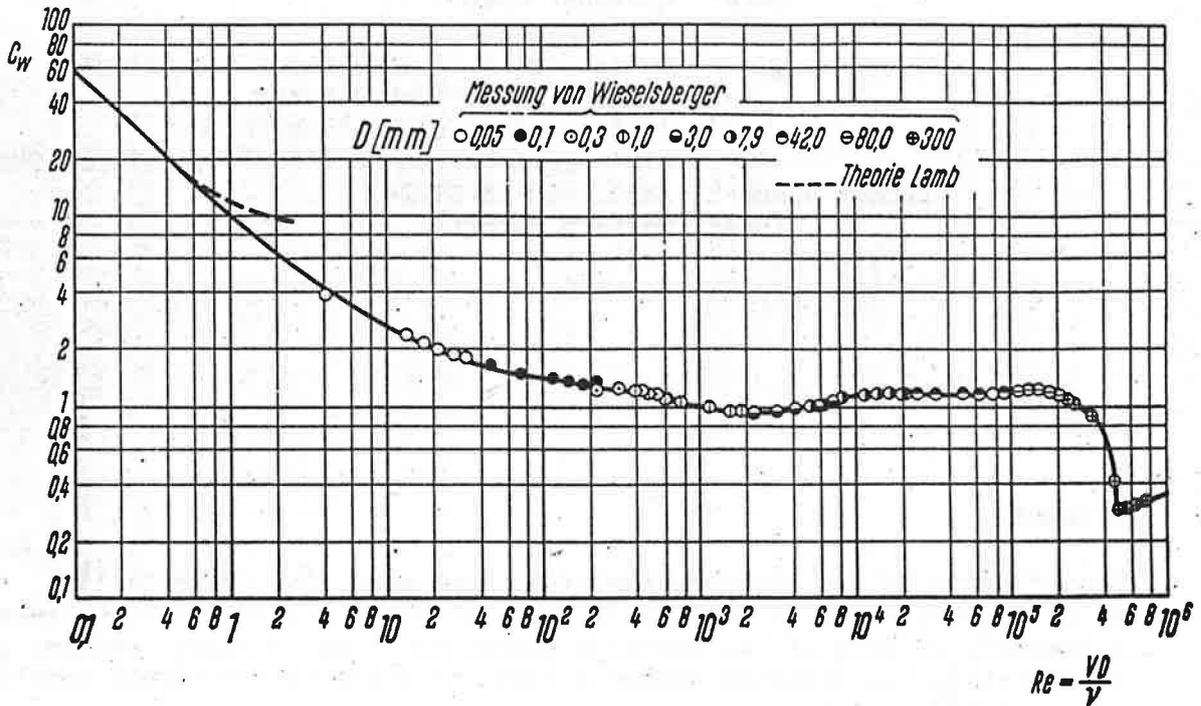
Fig. 1 Drag coefficient ( $C_w$ ) of circular cylinder as function of Reynolds number (based on diameter  $D$ ).
