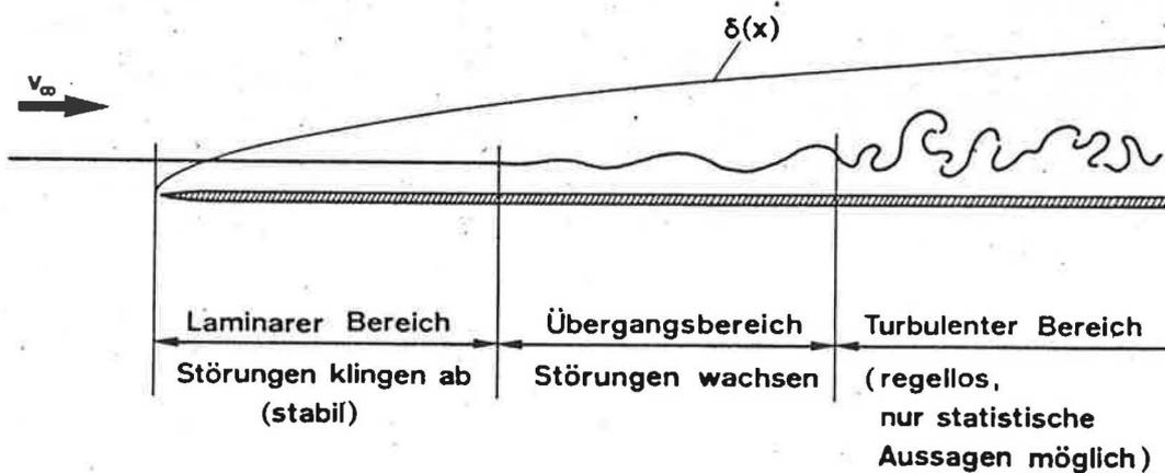
**Fig. 3** Boundary layer thickness,  $\delta(x)$ , and type of flow (laminar, transitional, turbulent) on a flat plate with sharp leading edge. Transition occurs at  $300,000 < Re_x < 3,000,000$ .
