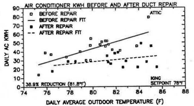
**Figure 11. Measured cooling energy use before and after repair of air distribution system leaks in six Florida homes.**
