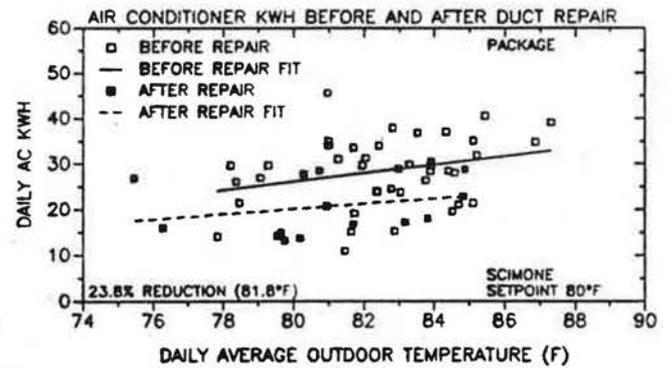
**Figure 10. Measured cooling energy use before and after repair of air distribution system leaks in six Florida homes.**
