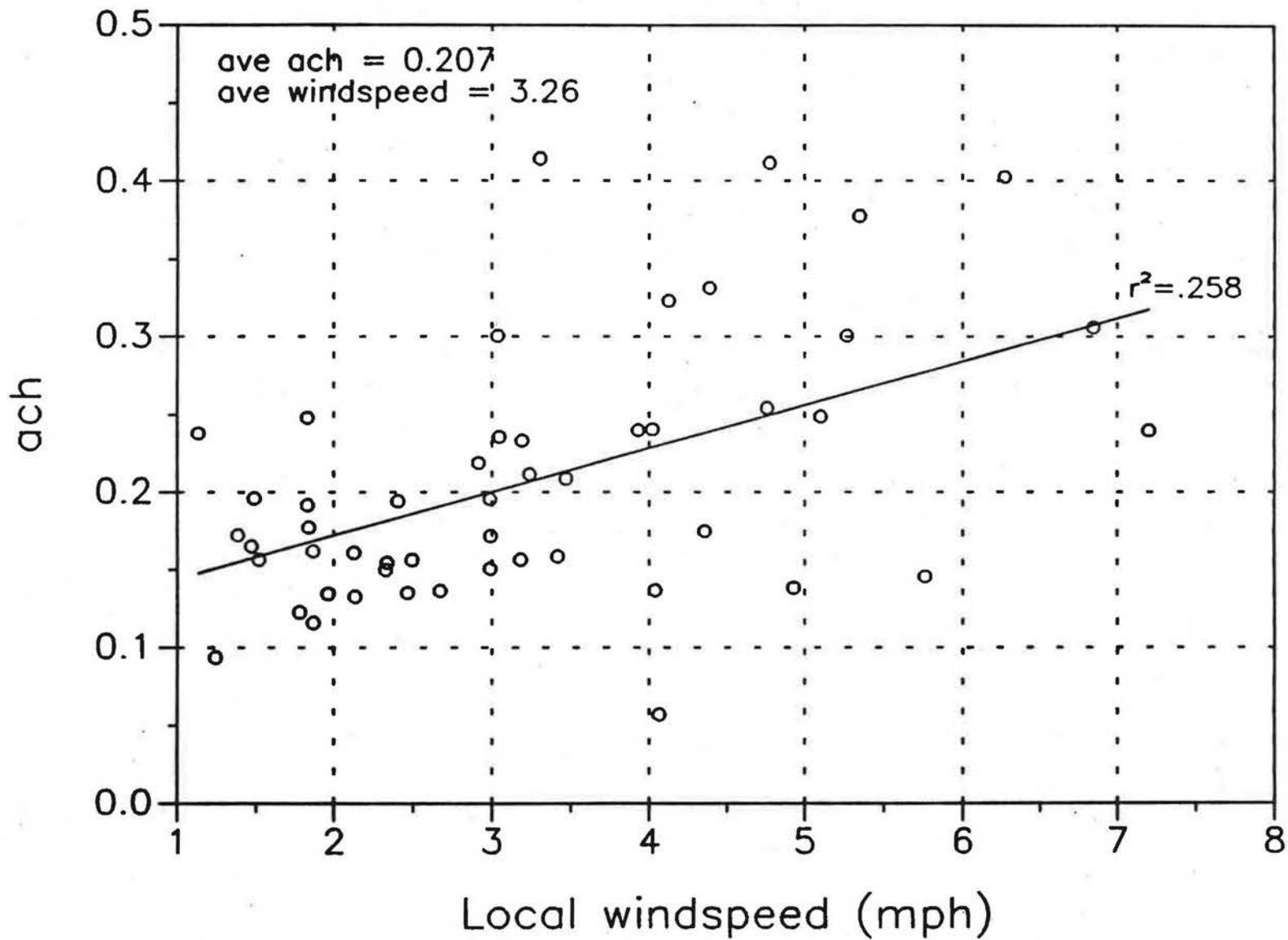
**Figure 3.** Tracer gas measured "natural" infiltration (air handler and all exhausts turned off) in 50 homes versus wind velocity measured by 7 foot tower on site. (Source: Cummings, Moyer, and Tooley, 1990)
