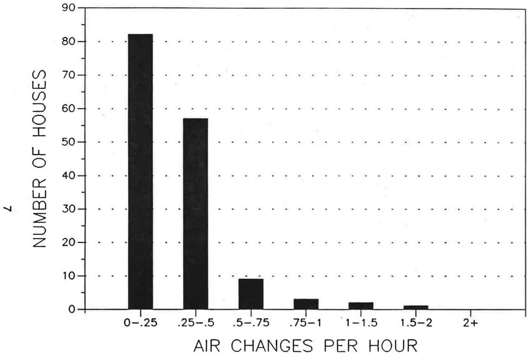
**Figure 1. Tracer gas infiltration rates in 154 homes with the air handler off. Average = 0.28.**
