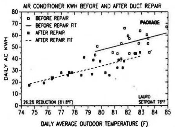
Figure 9. Measured cooling energy use before and after repair of air distribution system leaks in six Florida homes. (Source: Cummings, Tooley, Moyer, and Dunsmore, 1990)
