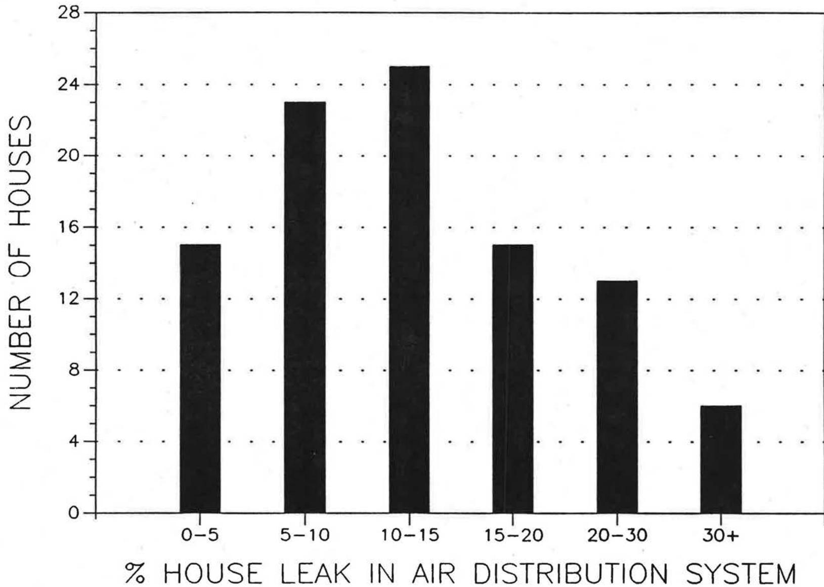
**Figure 6.** Percent of house air leakage at 50 pascals which is located in the air distribution system of 95 homes, determined by blower door. Average = 12.7%
