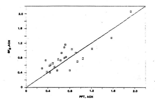
Figure 4. Correspondence between SF6 and PFT measurements of air infiltration rates for 24 homes.
