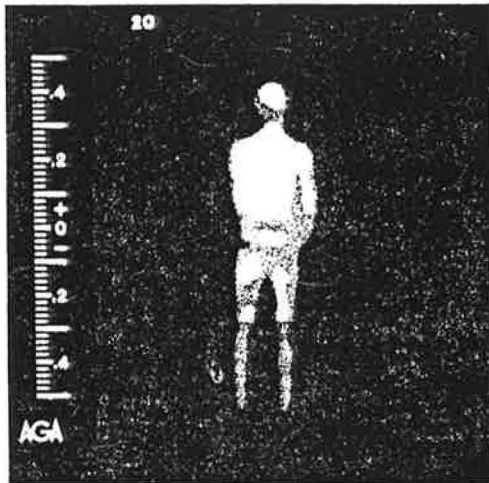
Fig. 18 IR-photo for the thermal manikin when surrounding temperature is equal to 22°C, skin temperature
