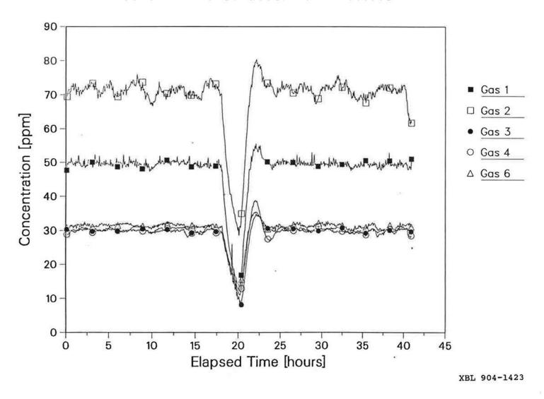
Figure 3b: shows the concentration of the gas being injected into zones 1-4 and 6.
