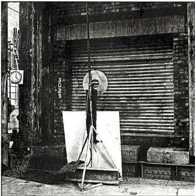
Moment of truth: but test conditions for smoke tightness of doors (BS 476) do not reflect real fire conditions with hot swirling gases.
