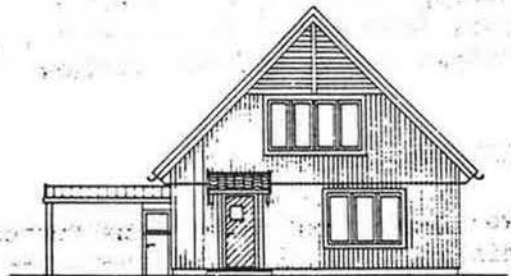
Figure 1. The picture above shows the house facades facing the street. The facades are of vertical wooden boarding. On the left, a cross-section of the house construction. The houses are to a fairly high degree prefabricated. The foundation elements, which are left in position, act as forms for the concrete slab which is cast on the spot. These foundation elements consist of a core of polystyrene foam surrounded by an outer layer of concrete reinforced with steel-fibre and glassfibre.
