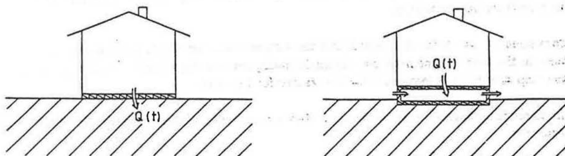
Figure 1: Heat loss Q(t) for a building with a foundation of the type slab on the ground and crawl-space.
