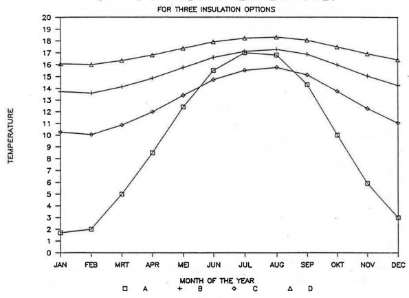
FIGURE 2 Crawl space temperatures as computed by the simplified spreadsheet model.
