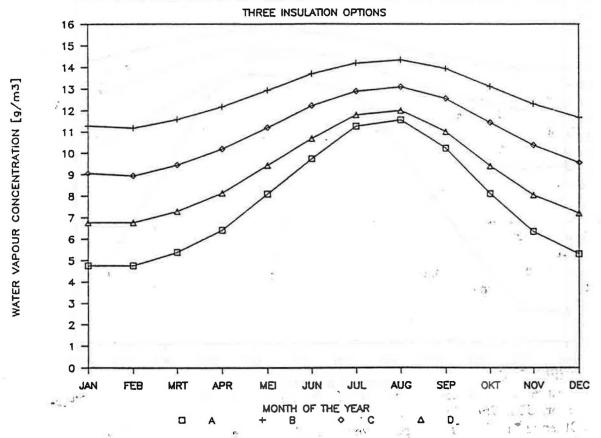
FIGURE 3 Crawl space water vapour concentrations as computed by the simplified spreadsheet model.
