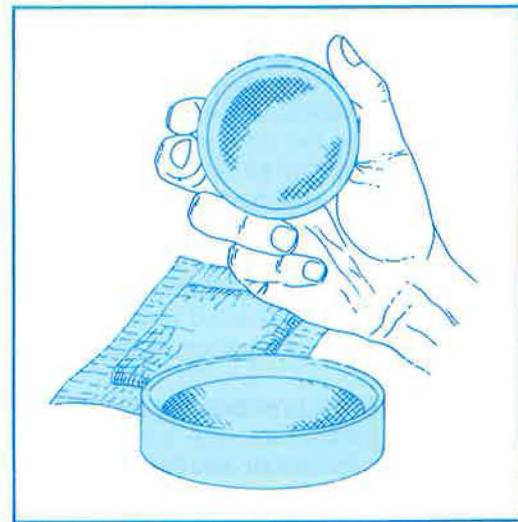
15. Activated charcoal measuring devices come in a variety of types. Shown here are a "tea-bag" collector and a charcoal canister.
