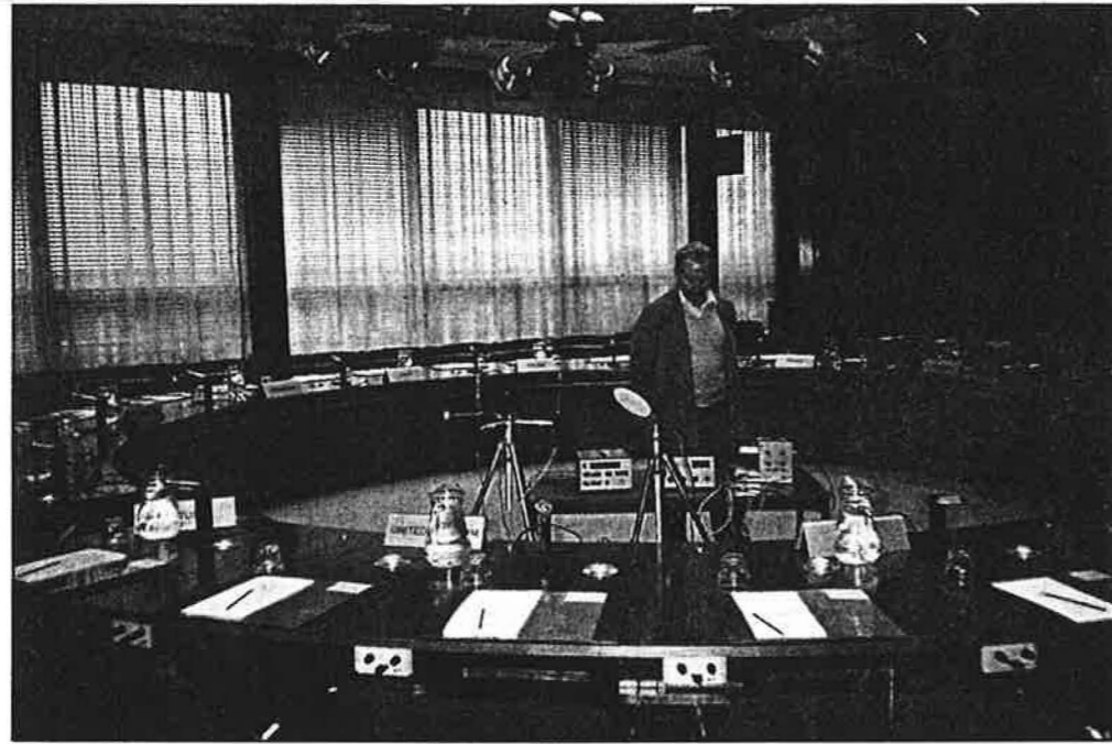
Above: A thermal environment survey was carried out by the investigating team, coupled with the distribution of questionnaires. Part of the problem was found to be the large areas of glazing, visible in the background.
