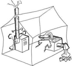
referred to as the House Depressurization Limit (HDL). When a house exceeds the HDL, the potential exists for prolonged start-up spillage or continuous spillage or backdrafting whenever the furnace operates.
