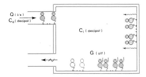
Fig. 1. A space with total pollution sources G and perceived air quality  $C_i$ , ventilated by a flow of outdoor air with the air quality  $C_0$ .
