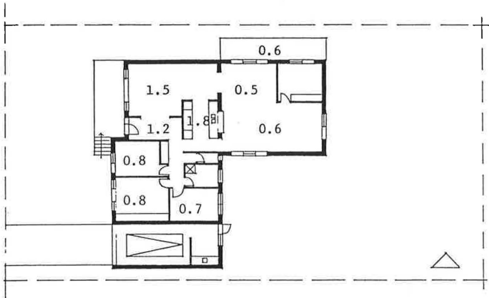
Fig. 3. Plan of house 2. MF readings with power on are shown in mG.
