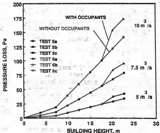
**Figure 6** Pressure drop distribution: with or without occupant simulation (closed treads, bottom injection)
