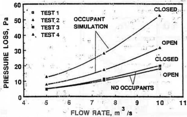
**Figure 5** Pressure drop between floors 7 and 8: effect of open and closed treads, with and without occupant simulation, bottom injection
