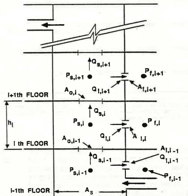
Figure 1 Stairshaft model for pressures and airflows
