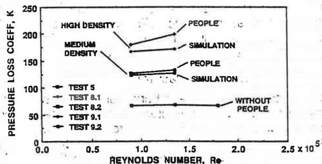
Figure 9 Validation of the simulation method by comparison with people tests (closed treads, bottom injection)
