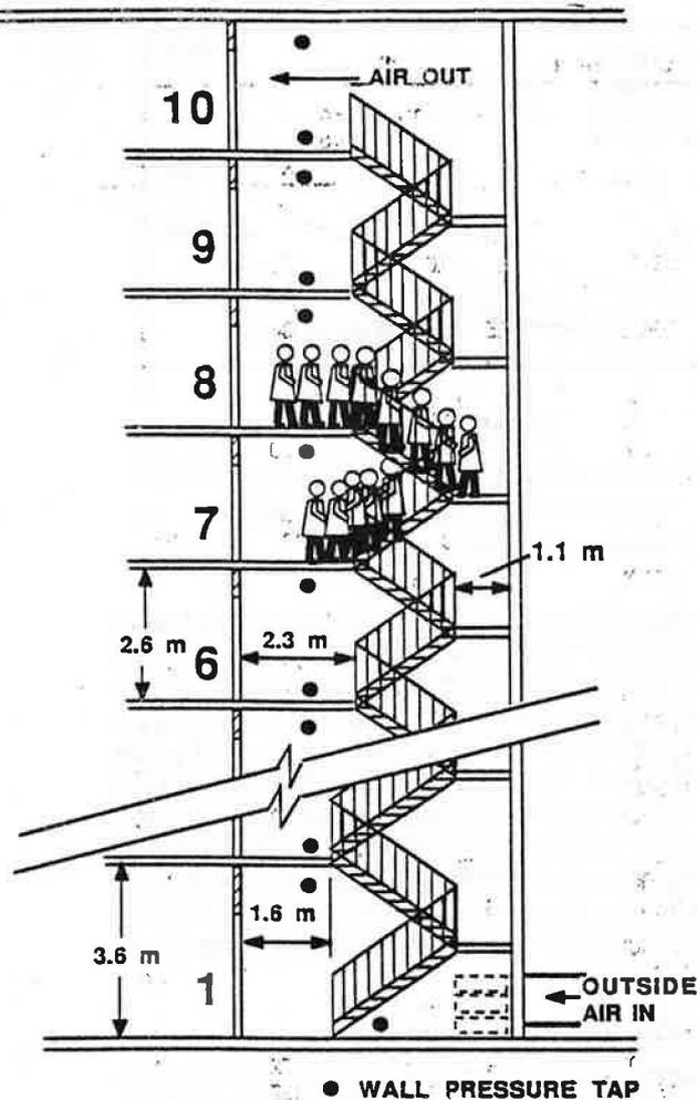
**Figure 2** Experimental stairshaft: location of pressure taps and occupant distribution
