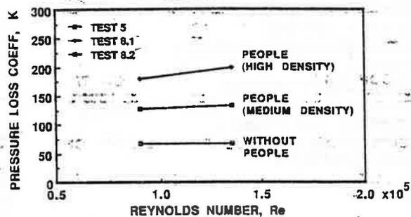
Figure 8 Flow resistance: effect of people at high and medium occupant densities (closed treads, bottom injection)
