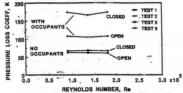
Figure 7 Flow resistance: effect of open and closed treads, with and without occupant simulation (bottom injection)
