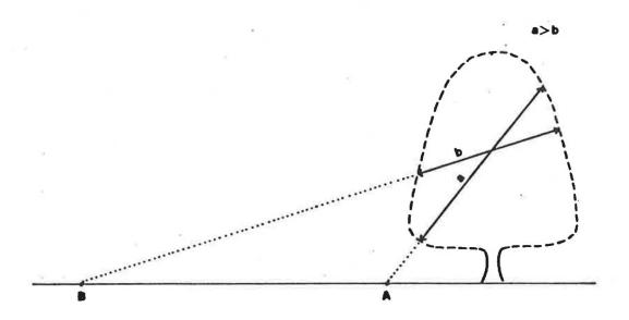
Figure 5. Diagram showing how the path length of solar radiation through a tree crown can be affected by angle of elevation. Light reaching point A has to travel further through the crown than that reaching point B.
