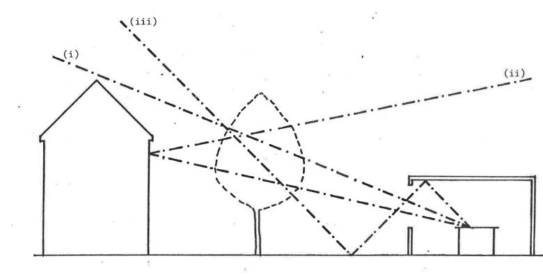
Figure 1. The three components of the daylight factor (i) sky component (ii) externally reflected component (iii) internally reflected component. All three components can be reduced by the presence of a tree.
