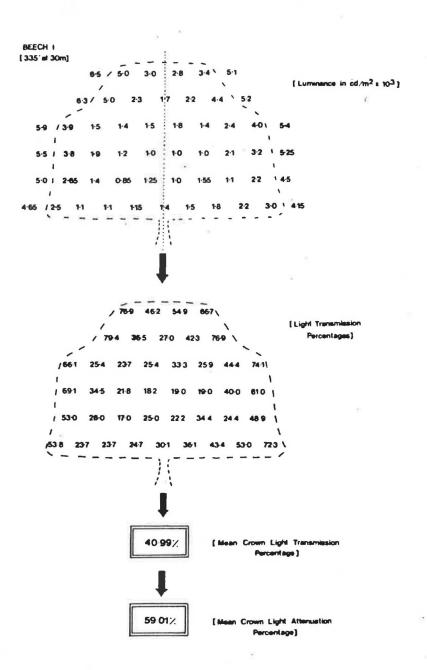
Figure 3. An example of the transformation of a set of measurements of luminous intensity into mean attenuation percentage.
