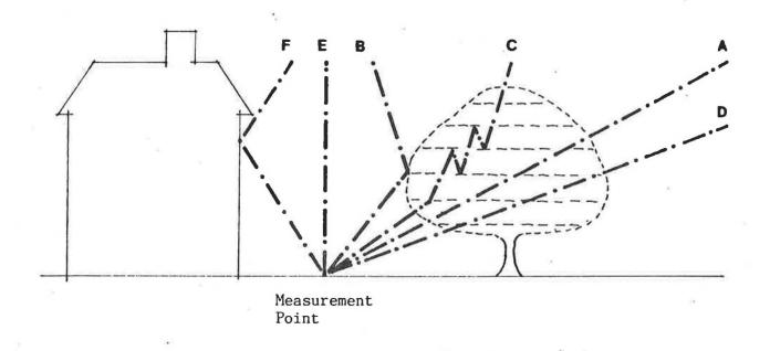
Figure 2. Possible pathways by which diffuse radiation can reach a measurement point.
