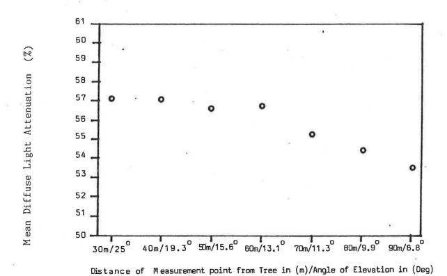
Figure 4. Graph showing the effect of the distance of the measurement point from the tree (thus angle of elevation of the tree) on diffuse light attenuation.
