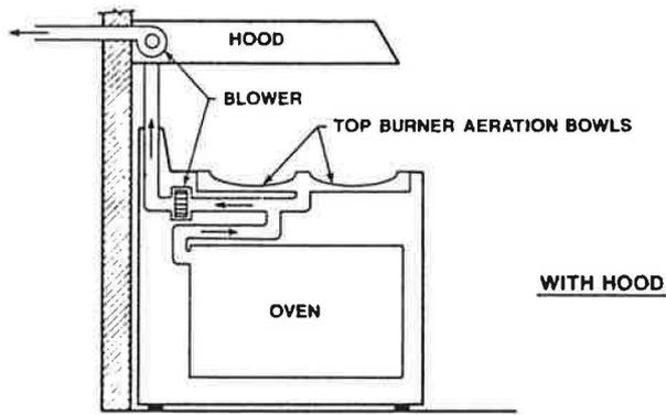
**Figure 9** Fully vented range installation configurations
