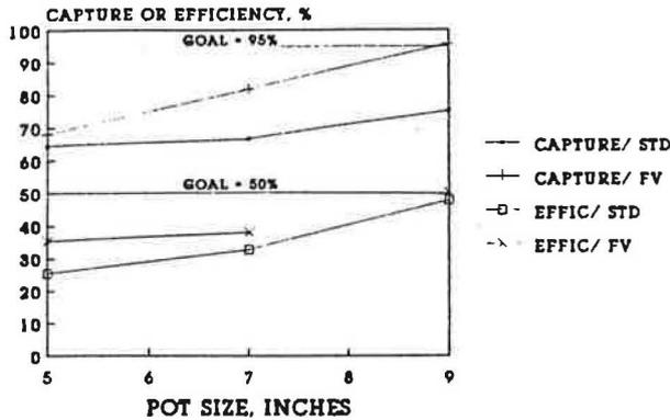
**Figure 11** Results of testing full vented and standard range with various size pots
