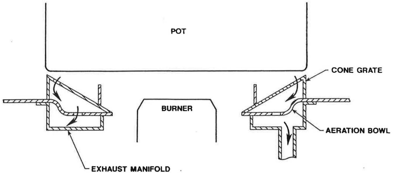
Figure 7 Cross-section of burner/aeration bowl with "cone" grate and exhaust manifold.
