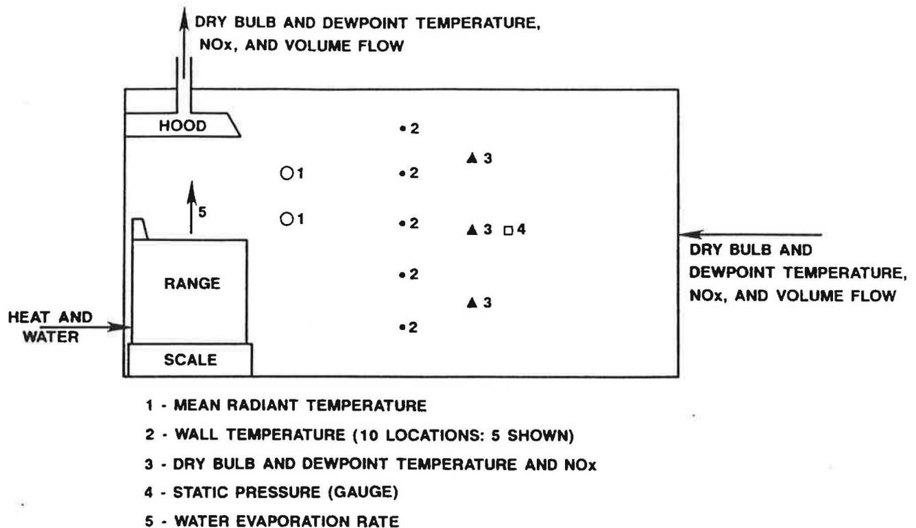
**Figure 4** Schematic of RVTC
