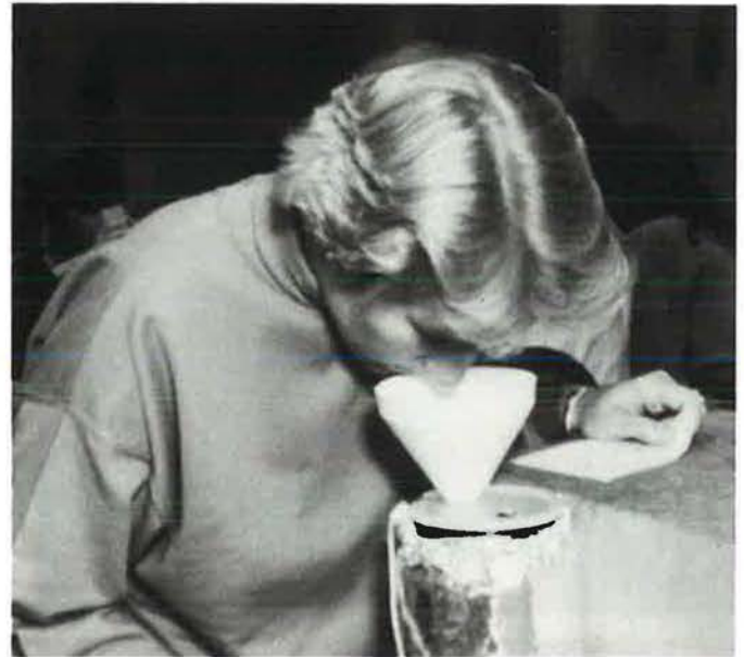
fig.3 One of the judges perceiving the air quality coming out of the sniffing instrument
