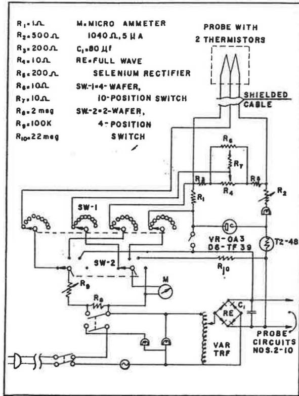
FIG. 2—SCHEMATIC WIRING DIAGRAM OF POWER SUPPLY, THE METERING CIRCUIT AND ONE OF THE PROBE CIRCUITS
