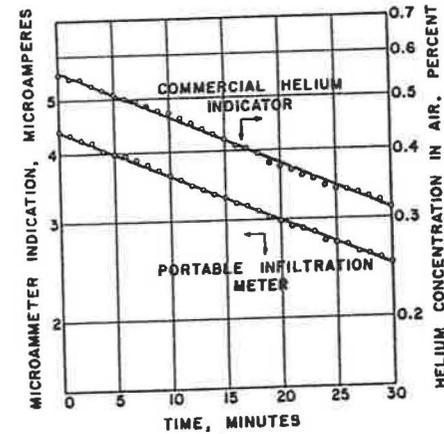
FIG. 3—DECAY CURVES OF PORTABLE INFILTRATION METER AND COMMERCIAL HELIUM INDICATOR
