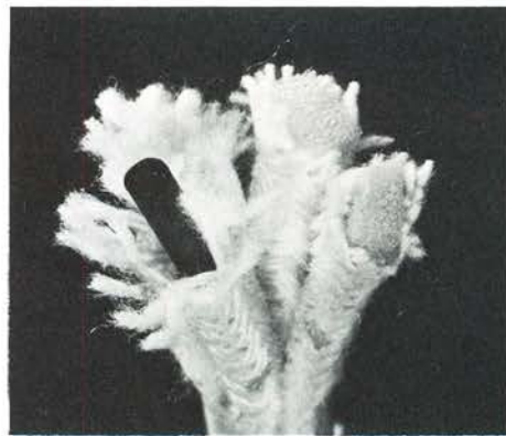
Spun fibre strips with core of foamed plastic and porous rubber.
