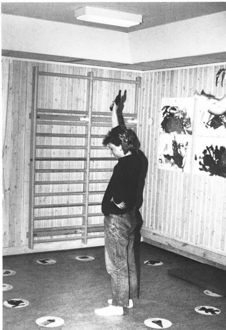
Children's games are often noisy; sound-damping wall panels and suspended ceilings give a better environment. Here, the reverberation time in a playroom is measured using a starting pistol. Photo: Johnny Andersson.
