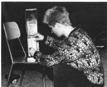
In the underfloor space of the day nursery, the air temperature and air humidity are registered using a thermohygrograph. Photo: Johnny Andersson.
